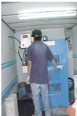
Fig 4.4.5c Conventional Compression Tester on Mobile Testing Laboratory
